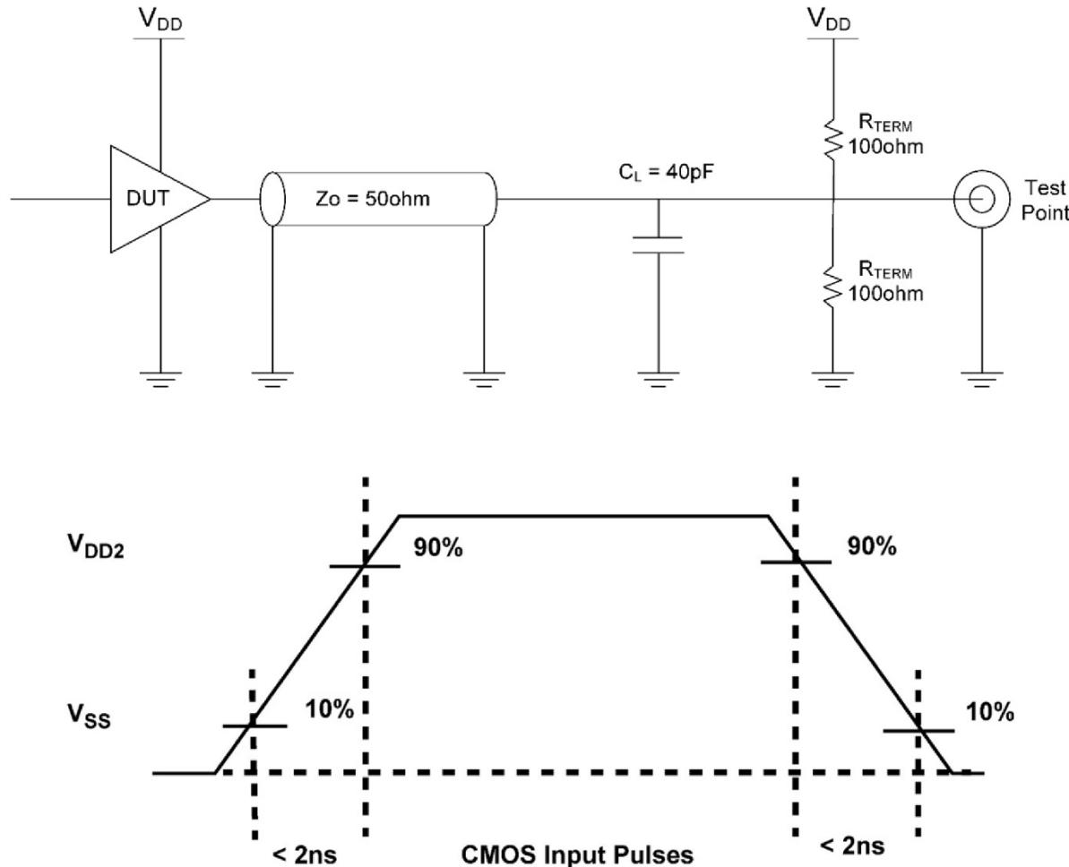
Figure 8. AC Test Loads and Input Waveforms
