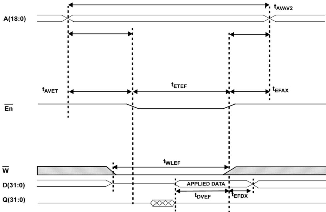
Figure 4b. SRAM Write Cycle 2: Enable - Controlled Access
