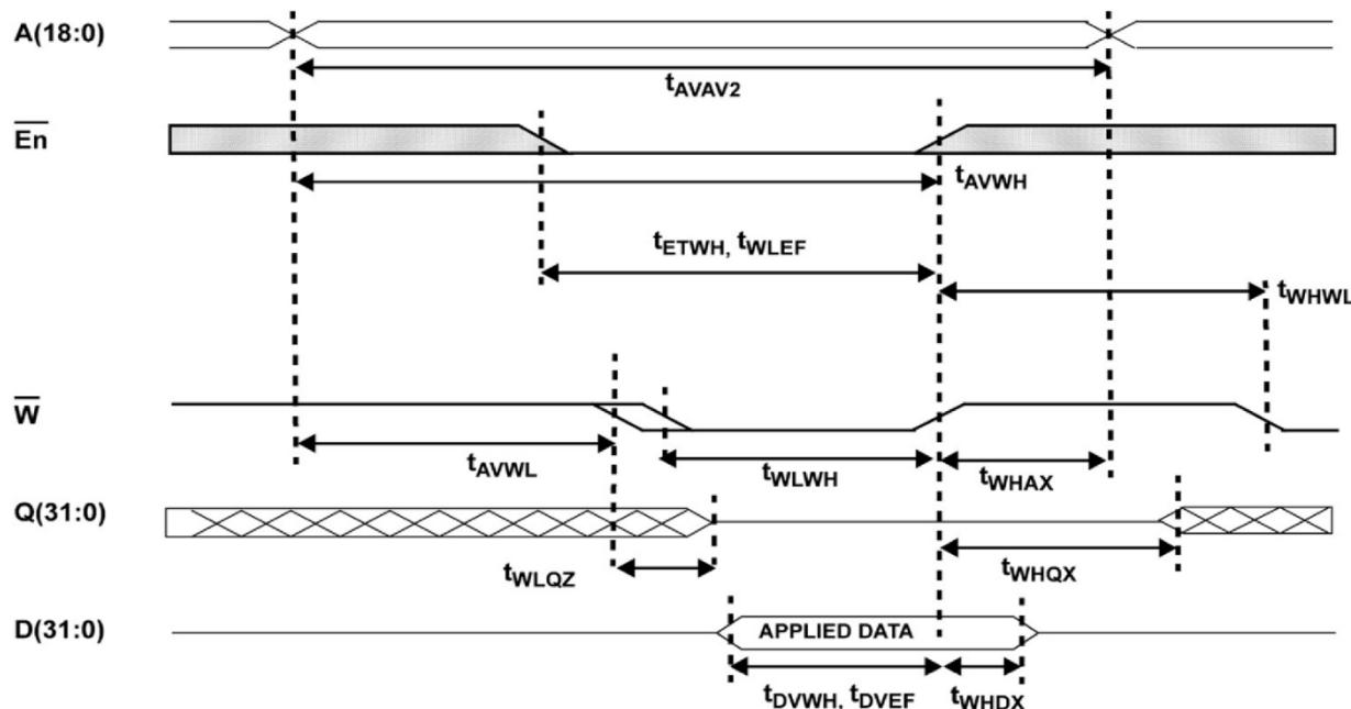
Figure 4a. SRAM Write Cycle 1:  $\overline{W}$  - Controlled Access
