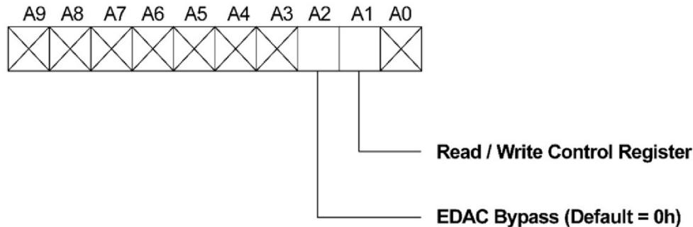
Figure 6. (Even Die Numbers (E2, E4, E6, E8 Chip Enables) EDAC Control Register
