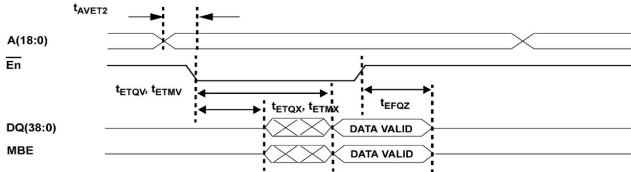
Figure 3b: SRAM Read Cycle 2: Chip Enable Access
