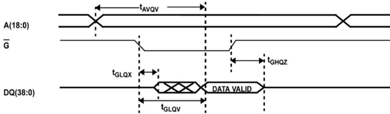
Figure 3c: SRAM Read Cycle 3: Output Enable Access
