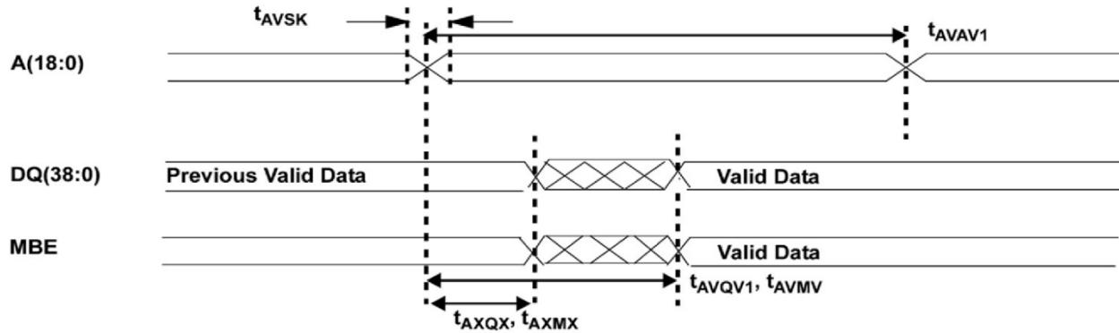
Figure 3a: SRAM Read Cycle 1: Address Access
