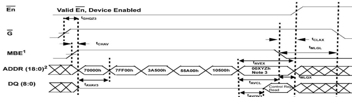
Figure 7a. Odd Die Numbers ( $\overline{E1}, \overline{E3}, \overline{E5}, \overline{E7}$  Chip Enables) EDAC Control Register Cycle
