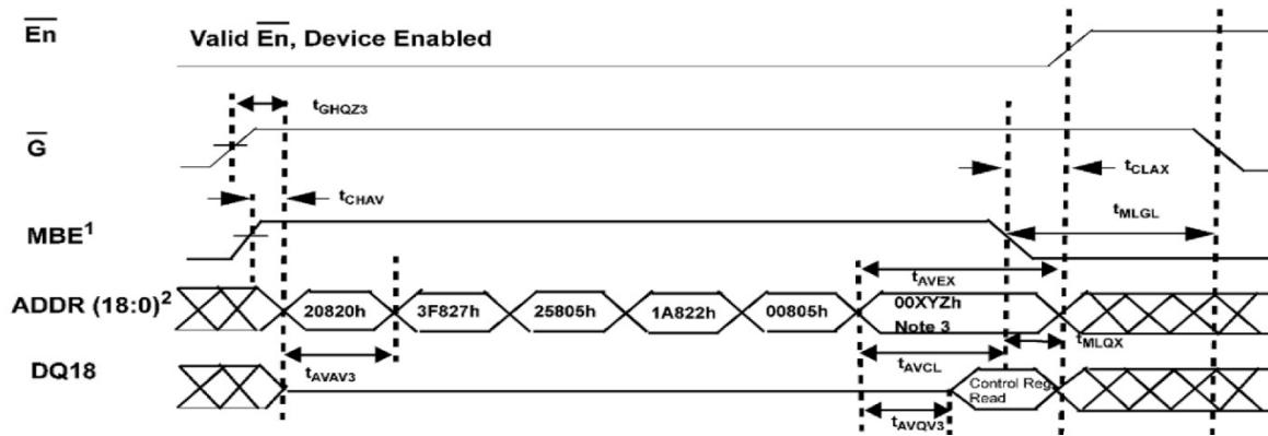
Figure 7b. Even Die Numbers ( $\overline{E2}$ ,  $\overline{E4}$ ,  $\overline{E6}$ ,  $\overline{E8}$  Chip Enables) EDAC Control Register Cycle
