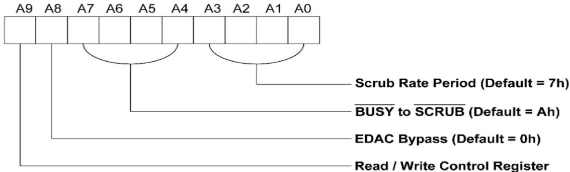
Figure 5. (Odd Die Numbers ( $\overline{E1}$ ,  $\overline{E3}$ ,  $\overline{E5}$ ,  $\overline{E7}$  Chip Enables) EDAC Control Register
