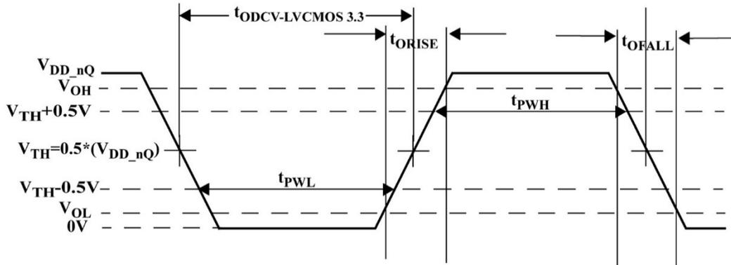
Figure 7a. +3.3V LVCMOS3.3/LVTTL Output Waveform
