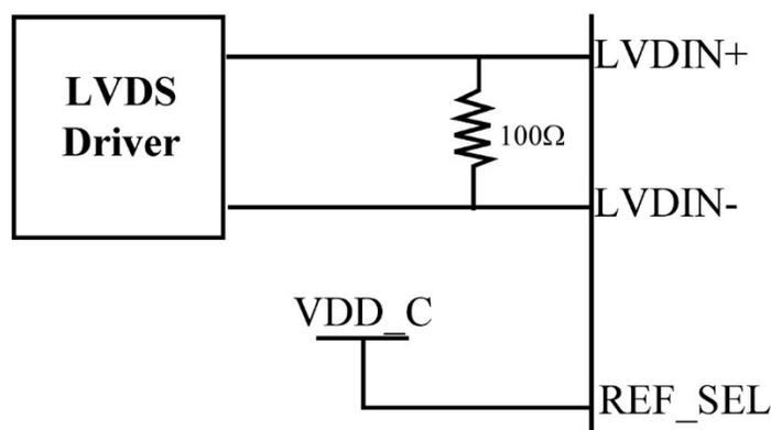
Figure 4. LVDS Reference Clock Interface
