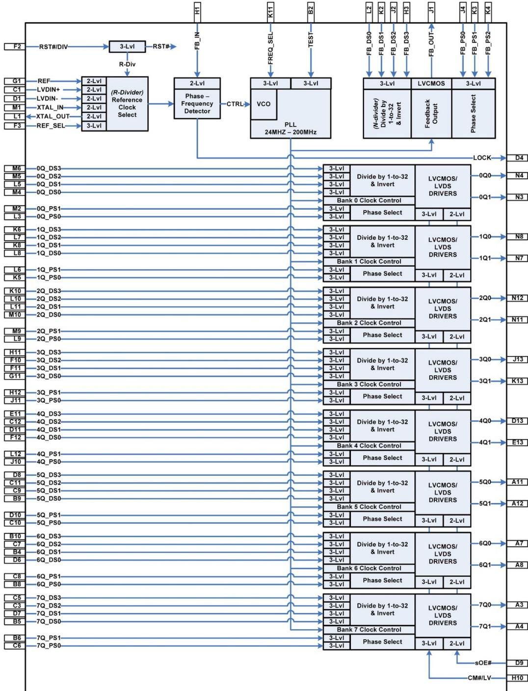
Figure 1. UT7R2XLR816 Block Diagram
