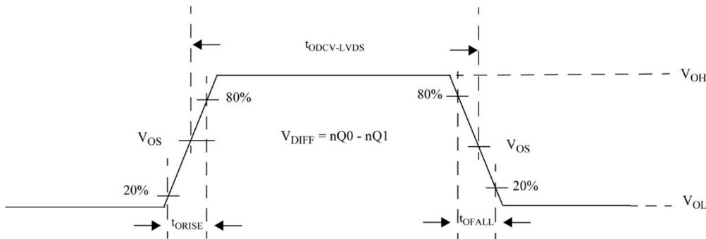
Figure 10. LVDS Driver Transition Time Waveform
