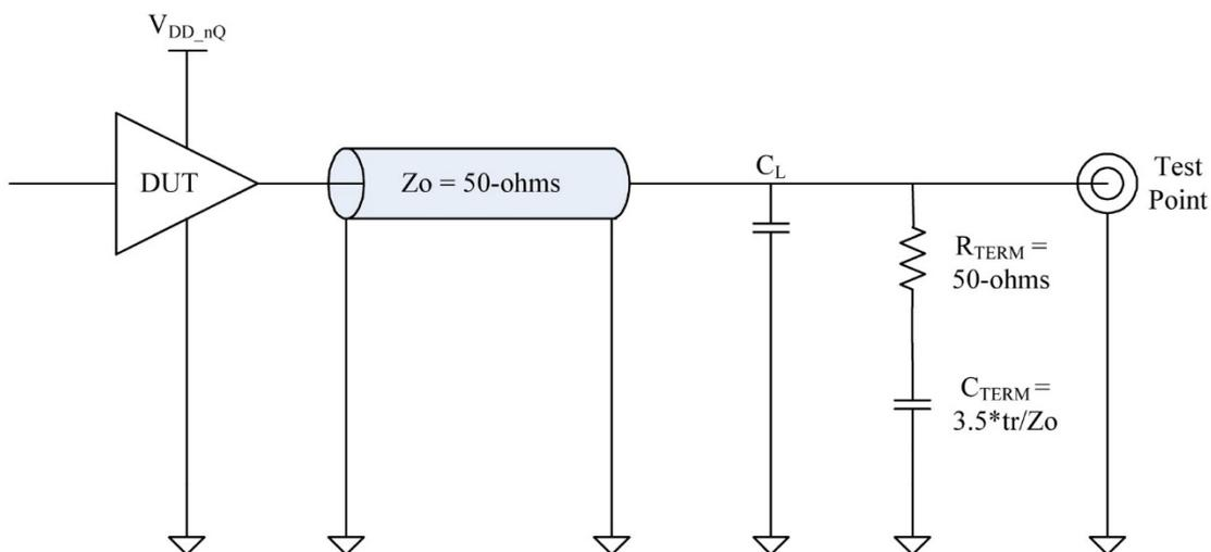
Figure 8c. AC Terminated LVCMOS/LVTTL Test Circuit
