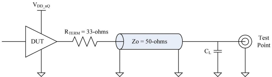
Figure 8a. Series Terminated LVCMOS/LVTTL Test Circuit
