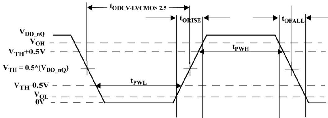
Figure 7b. +2.5V LVCMOS2.5/LVTTL Output Waveform
