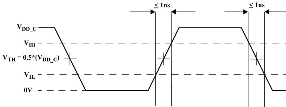
Figure 7c. LVCMOS3.3/LVTTL and XTAL\_IN Input Test Waveform
