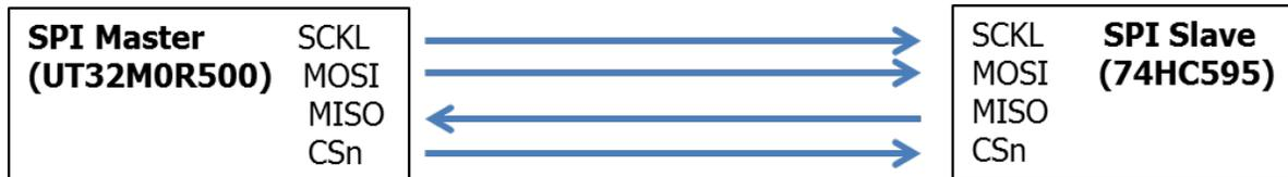
Figure 1: SPI master/slave communication
