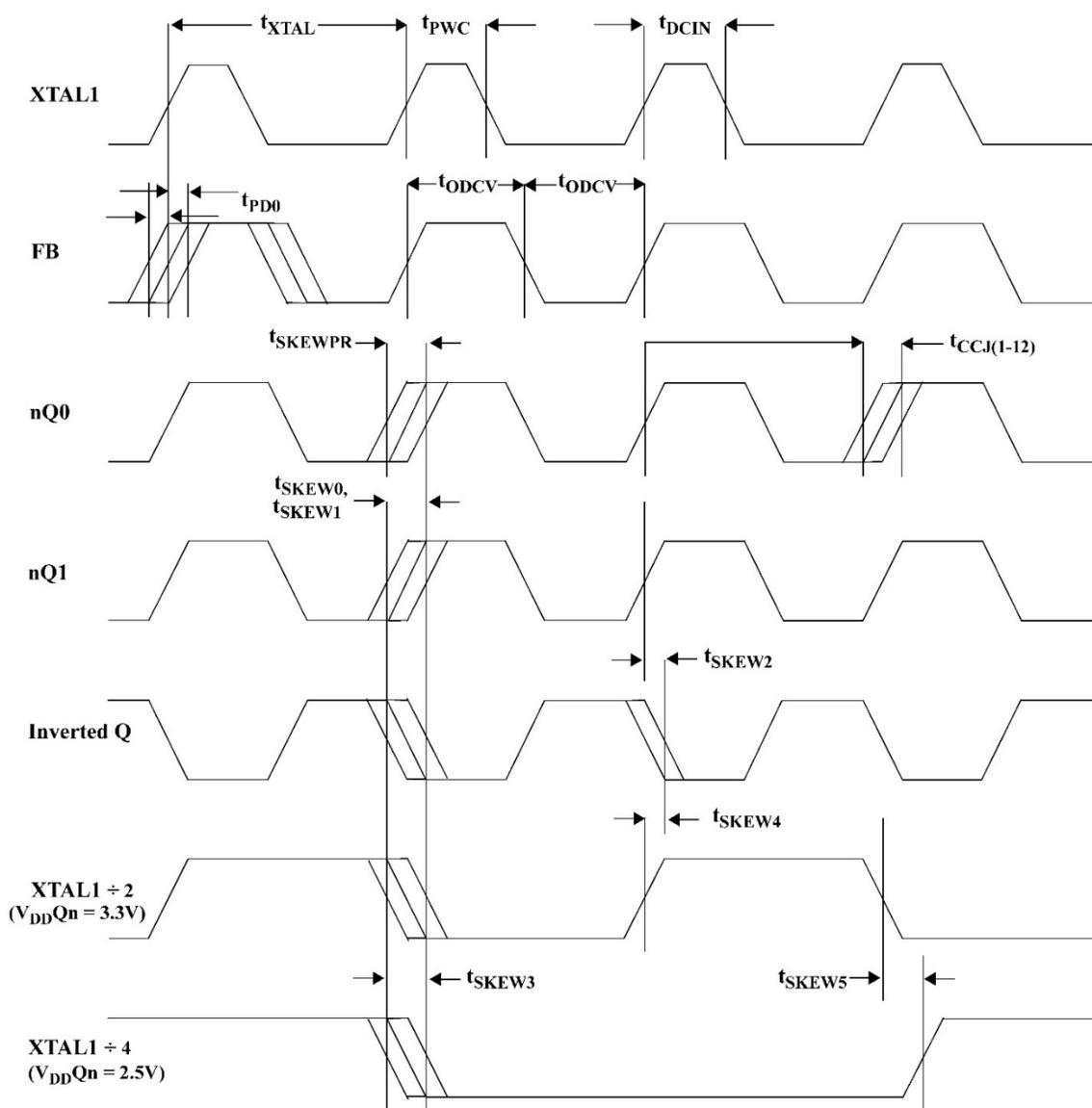
Figure 6. AC Timing Diagram
