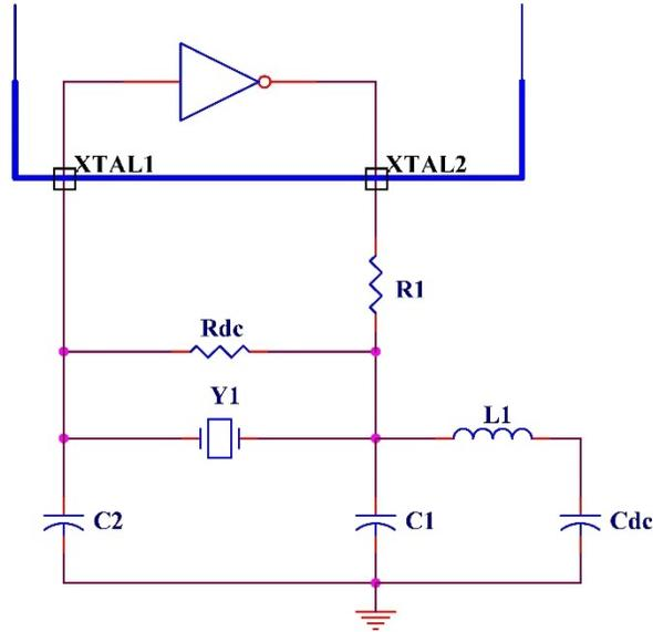
Figure 5. UT7R995C Pierce Crystal Oscillator with Tank Circuit
