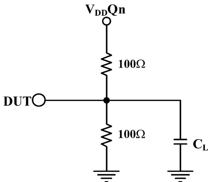
Figure 11. Clock Output AC Test Load Circuit
