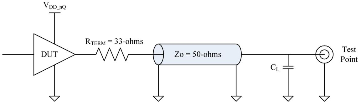
Figure 8A. Series Terminated LVCMOS/LVTTL Test Circuit
