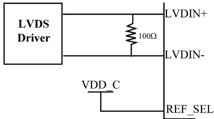
Figure 4. LVDS Reference Clock Interface
