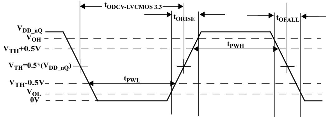
Figure 7A. +3.3V LVCMOS3.3/LVTTL Output Waveform
