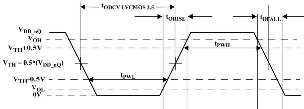
Figure 7B. +2.5V LVCMOS2.5/LVTTL Output Waveform
