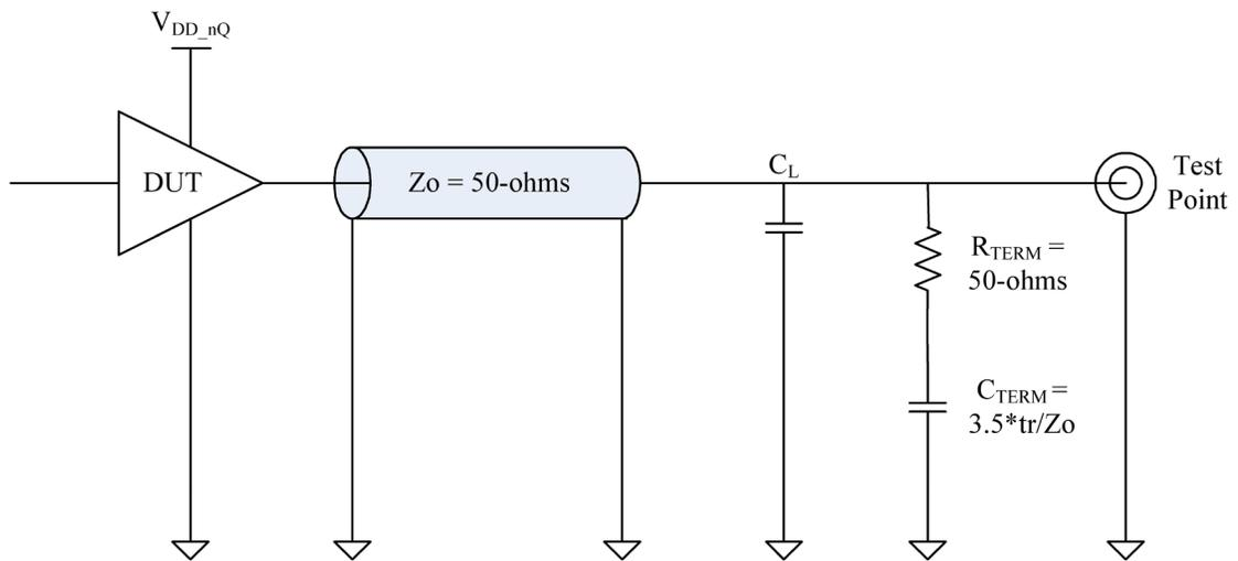
Figure 8C. AC Terminated LVCMOS/LVTTL Test Circuit
