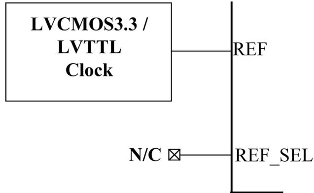
Figure 2. LVC MOS3.3/LV TTL Reference Clock Interface
