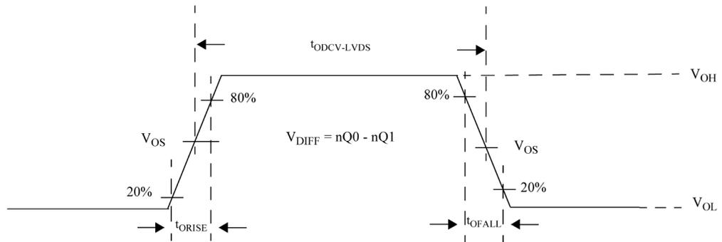
Figure 10. LVDS Driver Transition Time Waveform
