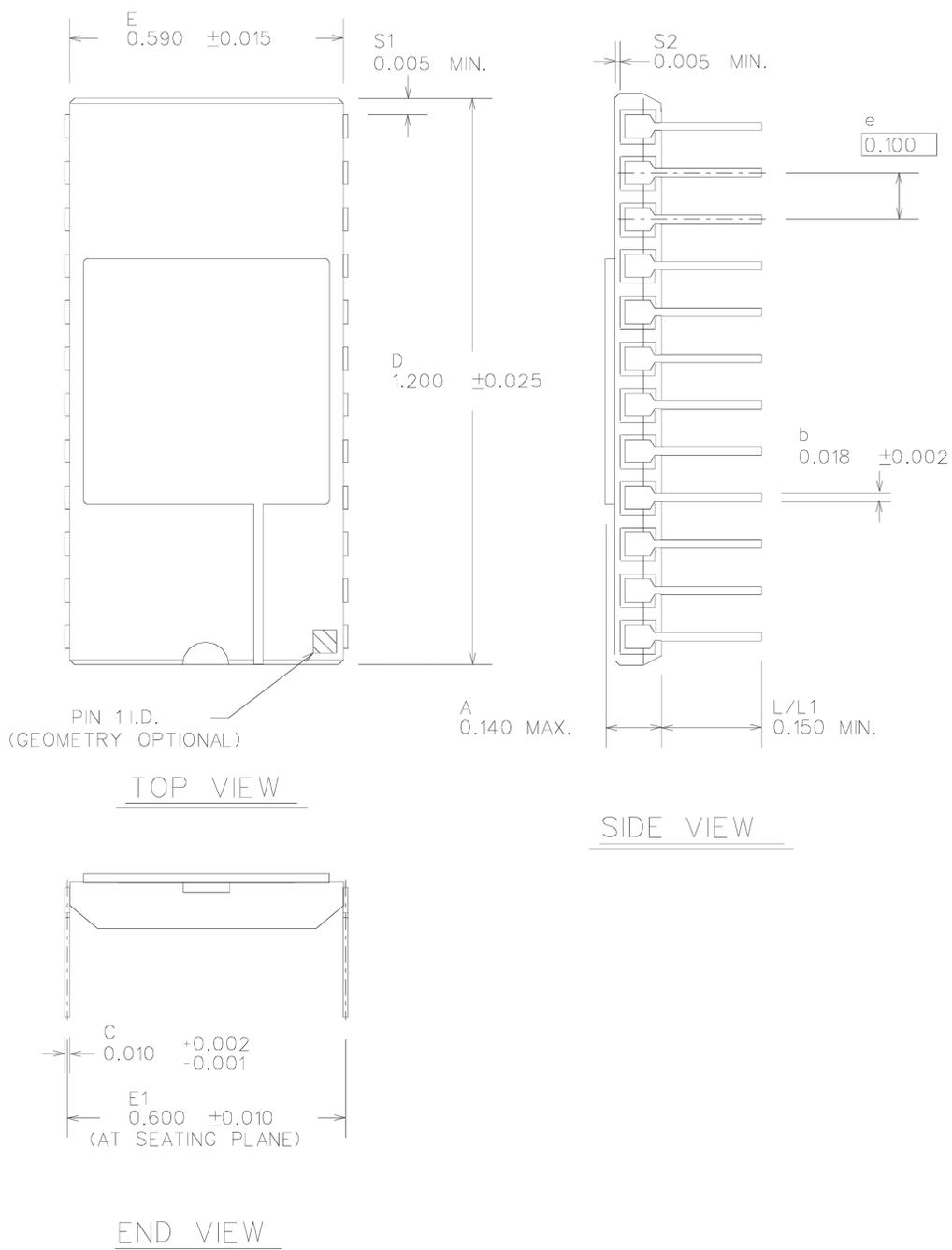
Figure 13. 24-Pin Side-Brazed DIP, Single Cavity
