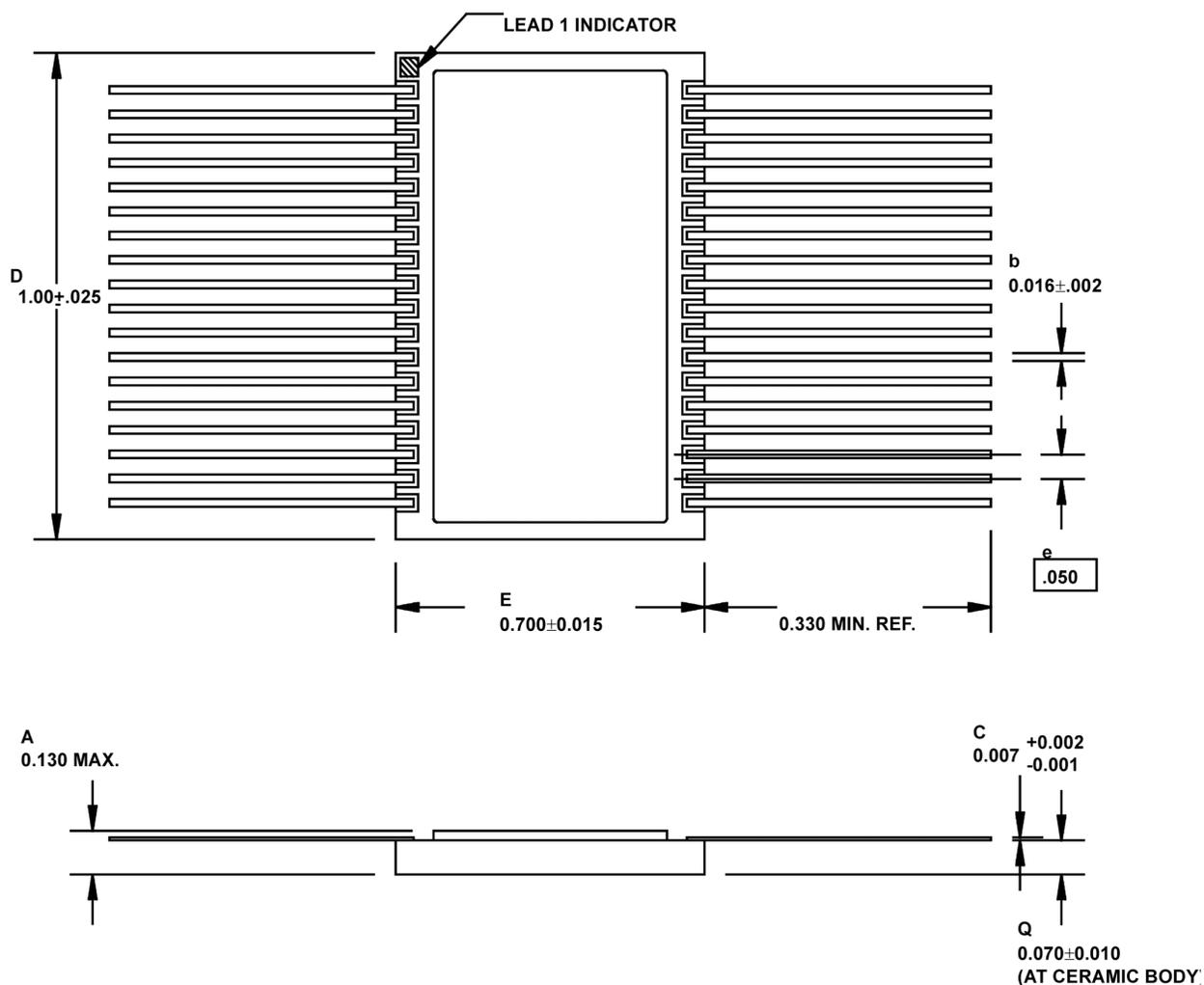
Figure 14. 36-Lead Flatpack, Dual Cavity
