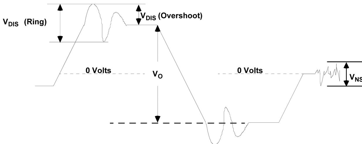
Figure 9. Transmitter Output Characteristics ( $V_{DIS}$ ,  $V_{NS}$ ,  $V_O$ )
