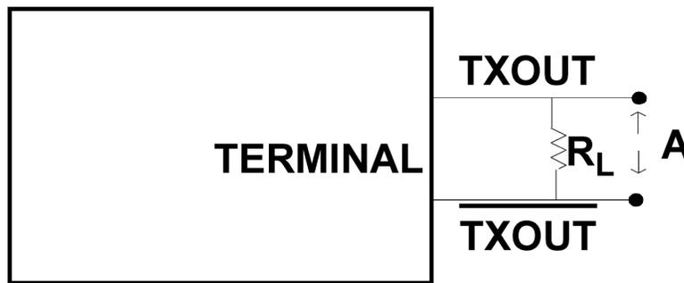
Figure 8. Transceiver Test Circuit MIL-STD-1553B
