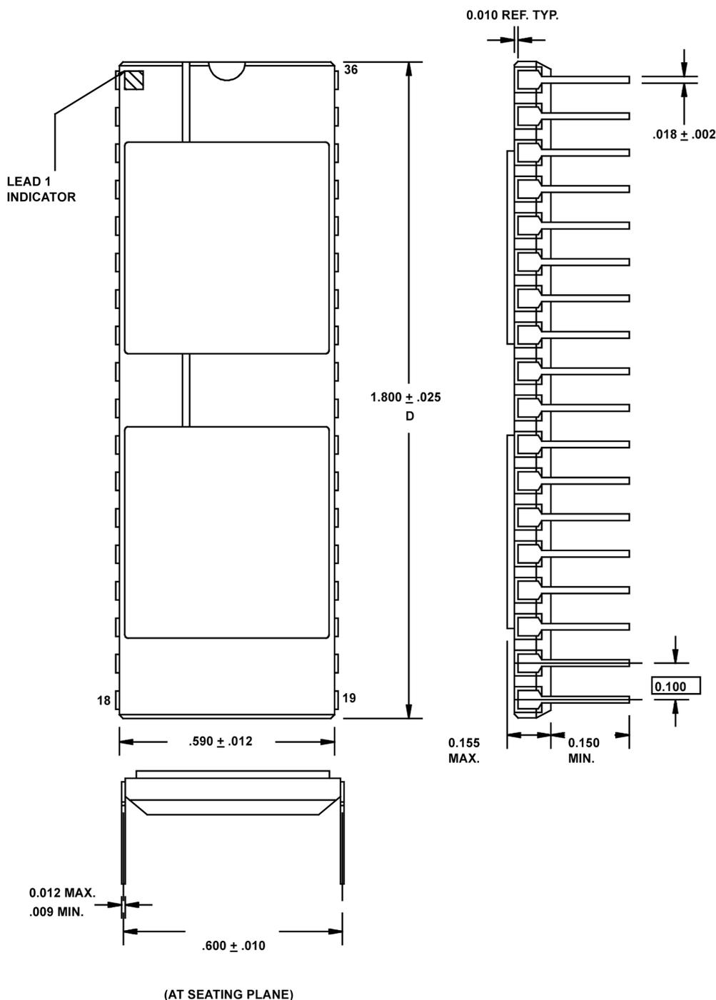
Figure 12. 36-Pin Side-Braced DIP, Dual Cavity
