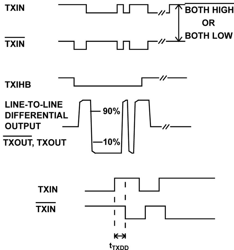
Figure 3. Typical Transmitter Waveforms
