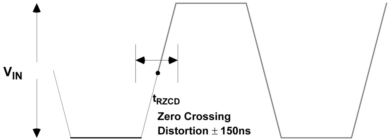
Figure 11. Receiver Input Zero Crossing Distortion ( $t_{RZCD}$ )
