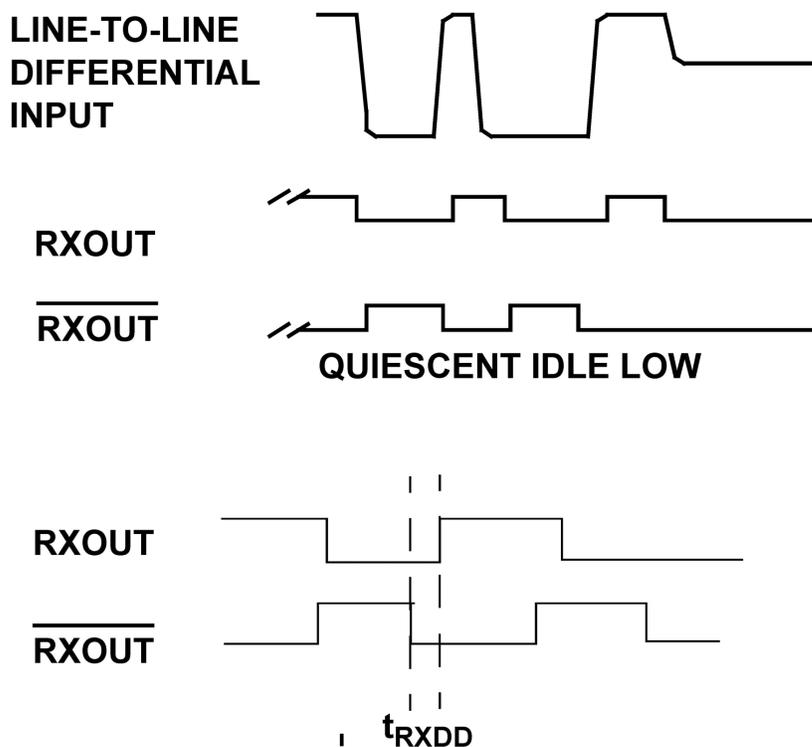
Figure 4. Typical Receiver Waveforms
