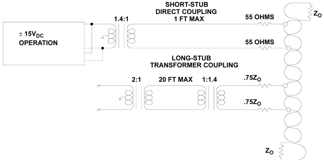
Figure 5. Bus Coupling Configuration
