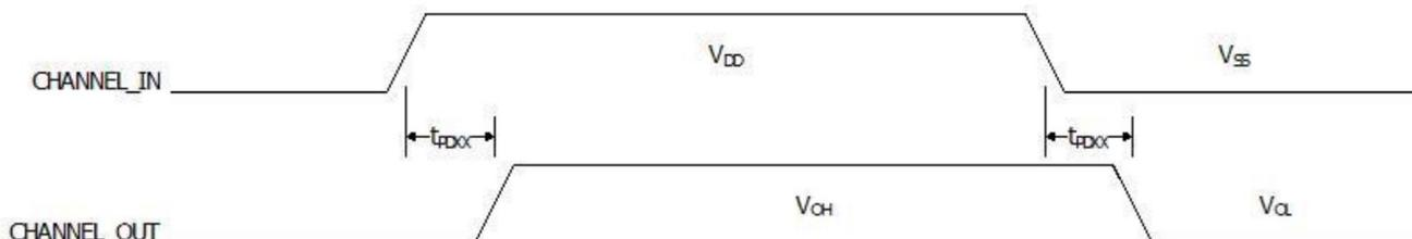
Figure 3: Channel Propagations Delay (/EN =  $V_{SS}$ )
