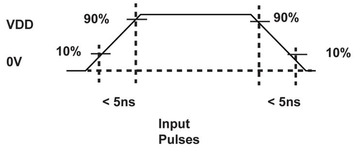
Figure 3. AC Test Loads and Input Waveforms
