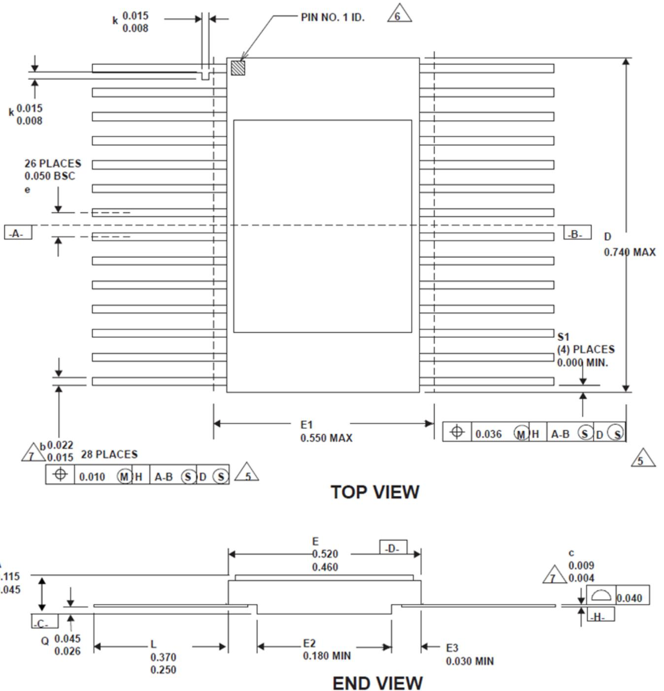
Figure 5. 28-Lead 50-mil Center Flatpack (0.490 x 0.74)
