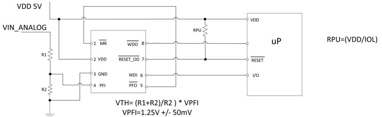
Figure 5. UT01VS50D Under Voltage Monitor and Detection
