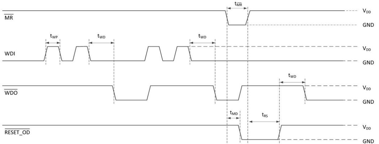
Figure 3.  $\overline{WDI}$  and  $\overline{WDO}$  timing waveforms. Reset externally triggered by  $\overline{MR}$
