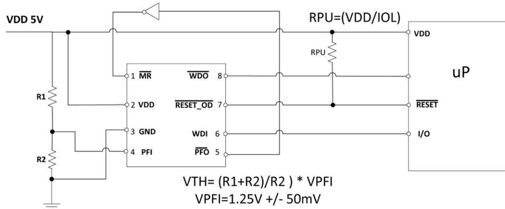
Figure 7. UT01VS50D Over Voltage Power Supply Monitoring and Reset
