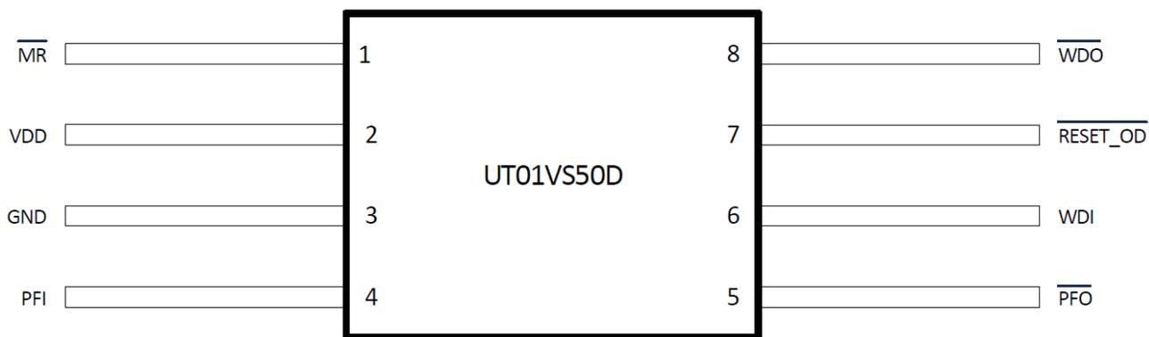
Figure 2. UT01VS50D Pin Configuration
