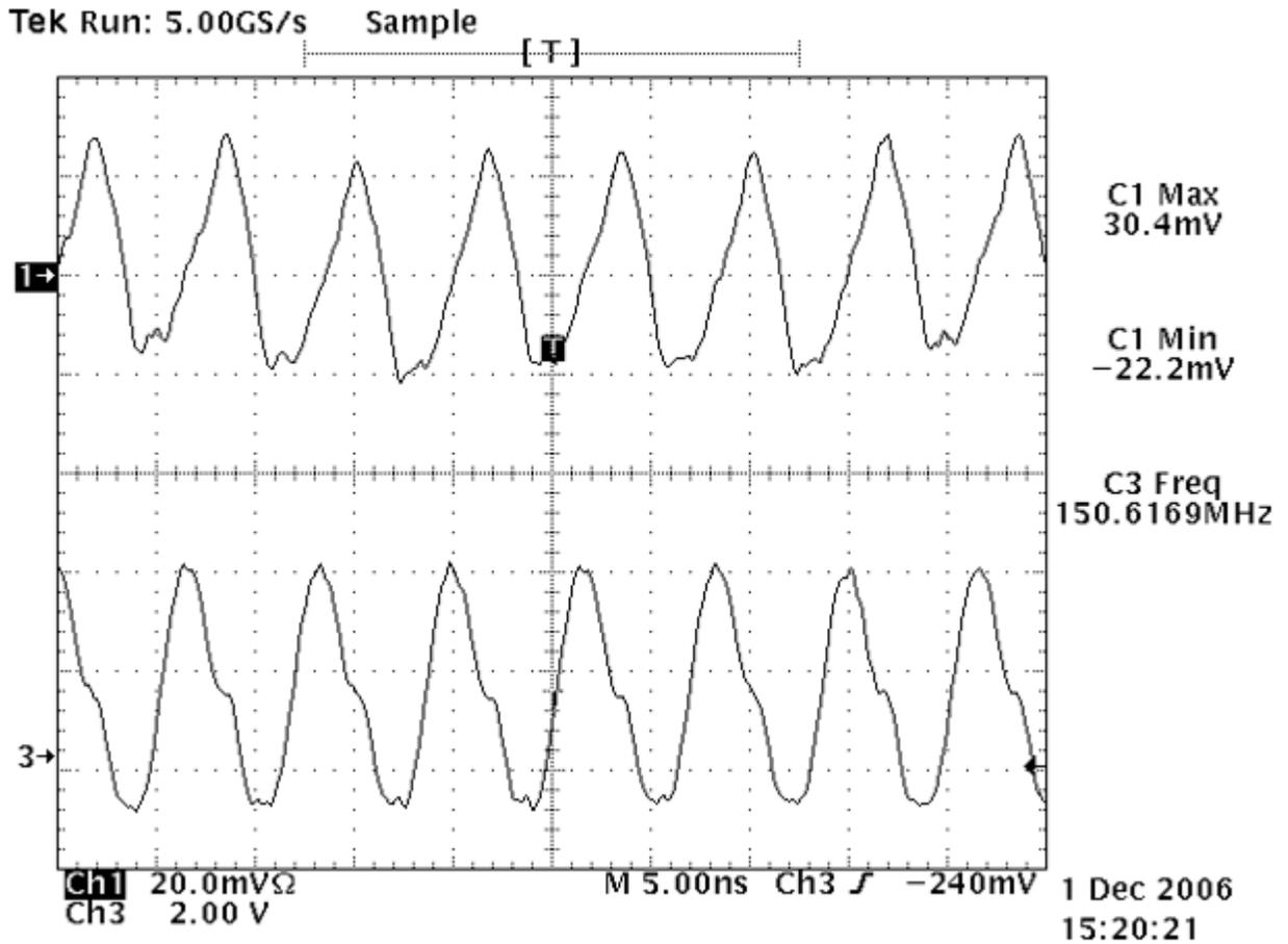
Figure 3.  $I_{DD}$  and Output Voltage for Channel 3Q0.
