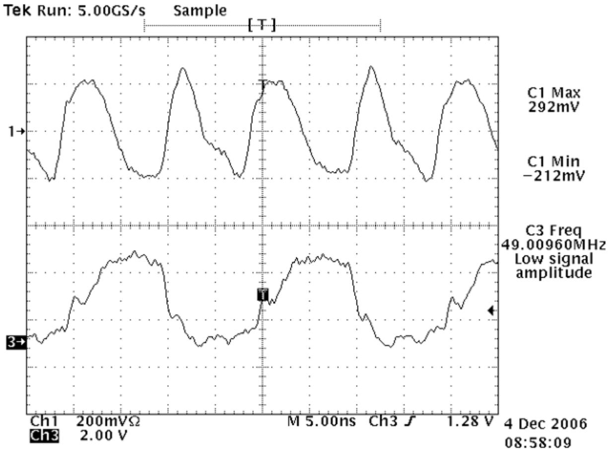
Figure 2.  $I_{DDQ3}$  and Output Voltage for Channel 3Q0.
