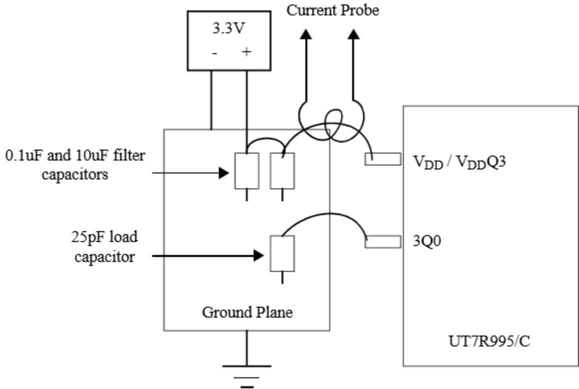
In the case where  $I_{DD}$  is being measured,  $V_{DDQ3}$  is connected normally through the power plane in the PCB. Like- wise, when  $I_{DDQ3}$  is being measured,  $V_{DD}$  is connected to 3.3V through the PCB. For the  $I_{DD}$  measurement, all  $V_{DD}$  pins are tied together.
