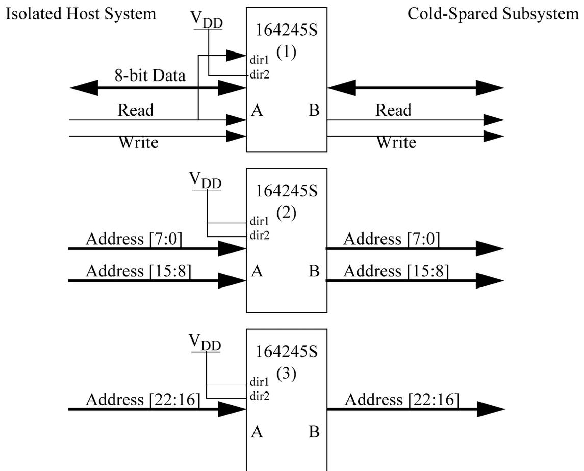
Figure 3. UT54ACS164245S Cold-Sparing Control
