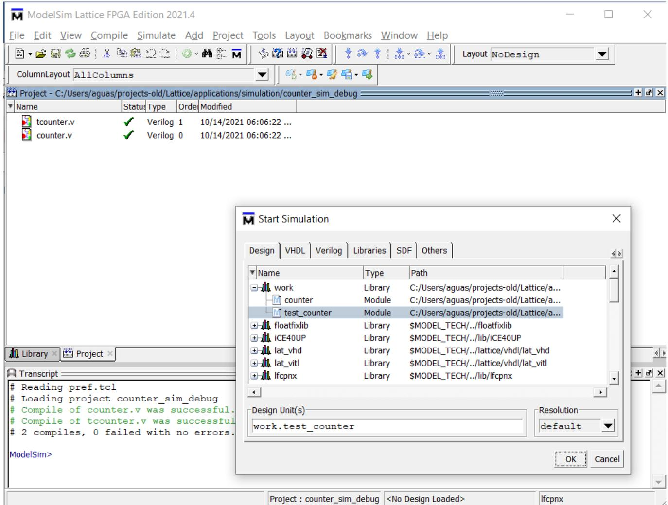
Figure 6: Starting a Simulation
